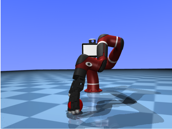
Fig. 2. Result of grasping with IK solver given target positions along the equator and downward orientation.
