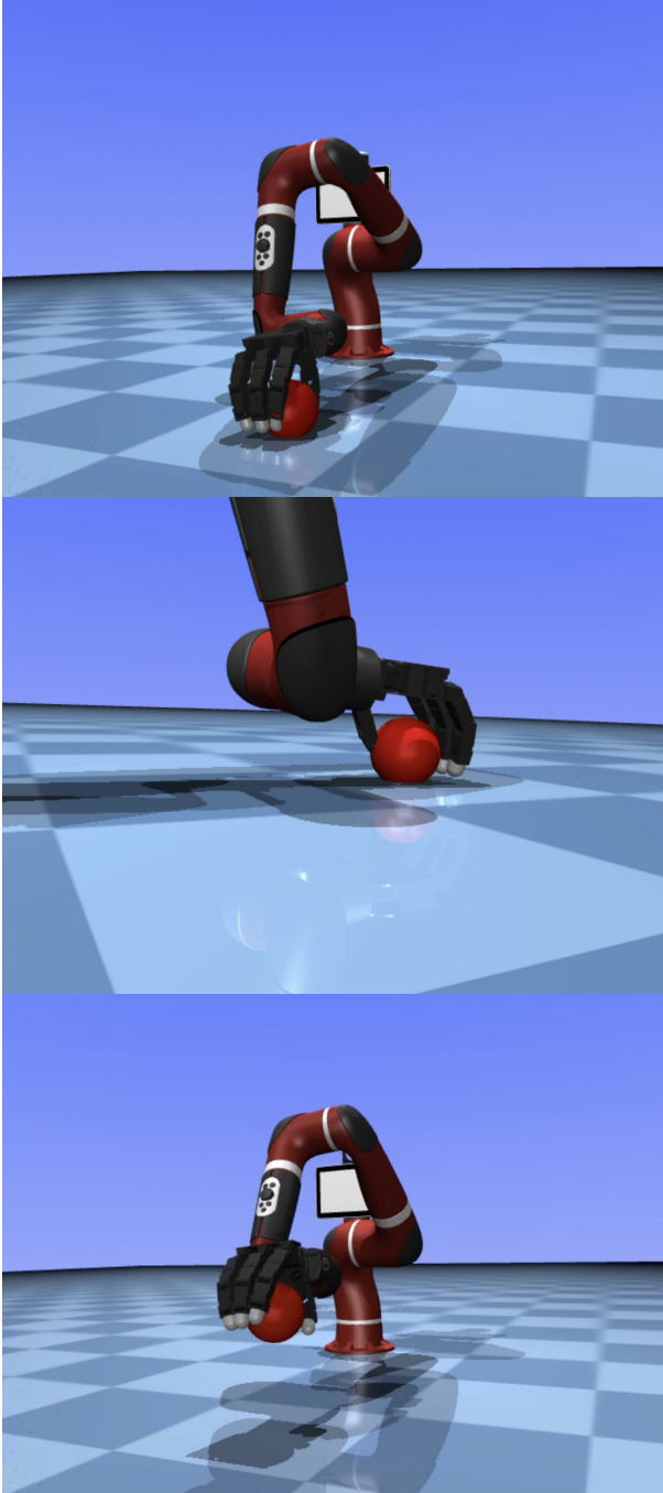
Fig. 4. Result of grasp synthesis. Top: front view of grasp. Middle: side view of grasp. Bottom: front view of grasp lifting the ball.
